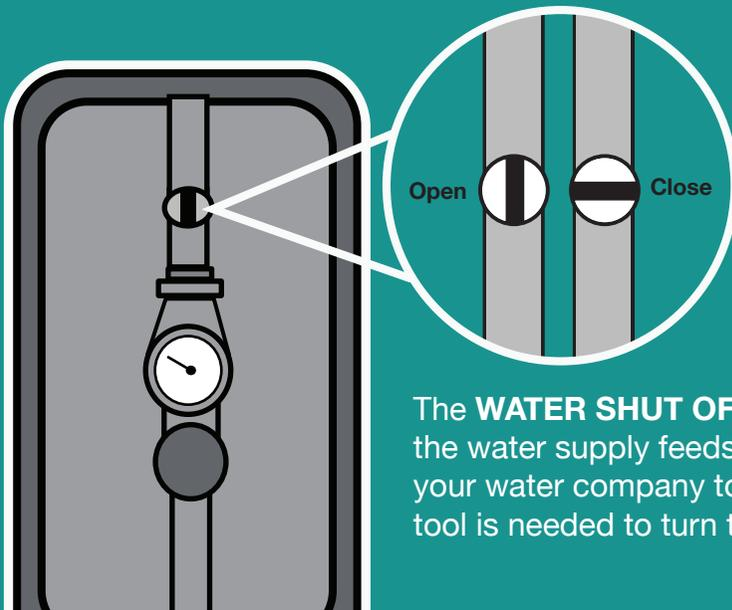
The **WATER SHUT OFF** valve is found where the water supply feeds the house. Check with your water company to determine if a special tool is needed to turn the valve.
