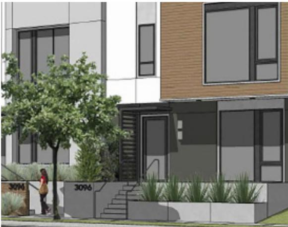
**a.** Small Lot Homes abutting a public right-of-way or private street shall orient the primary entryway (“front door”) toward the street or, where there is a physical site constraint, shall provide a clearly identifiable entry to the site from the street.
