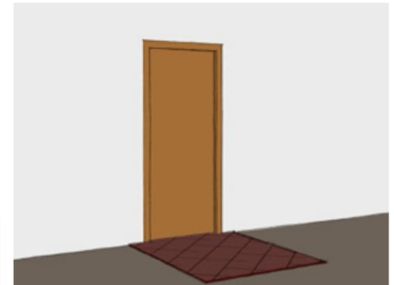
**vi.** The landing area shall be enhanced with unique paving material, texture, pattern, or color that is differentiated from the pedestrian pathway.
